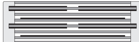
Extended double side metallized carrier film design with internal series connection and metallized film (series connection of 2 elements)
