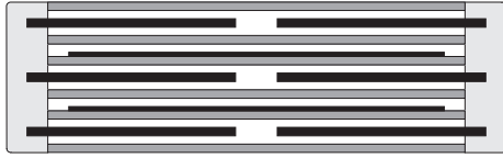
Extended foil design with internal series connection and metallized film (series connection of 2 elements)
