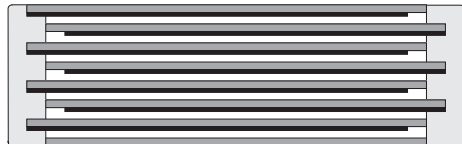
Extended metallized film design
