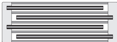
Extended double side metallized carrier film design
