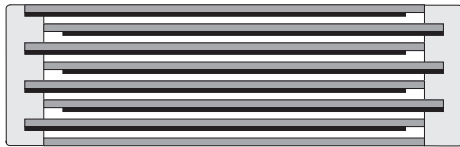
Extended metallized film design
